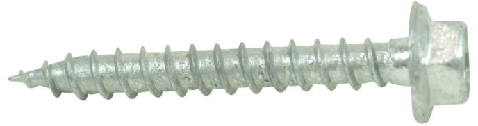
1192 4.. Fasthetsklasse 8.8 ISO 898/1 Rm = 800 N/mm2 Rp0.2 = 640 N/mm2 Varmforsinket 50 - 80 µm
